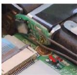
You have to detach the display carrier. Lift the display and unscrew the marked screws.
