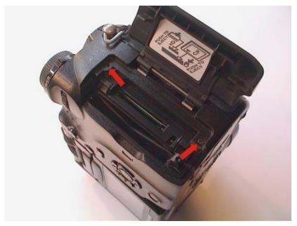
Put the camera on the left side and unscrew the two screws underneath the lid for the memory module.
