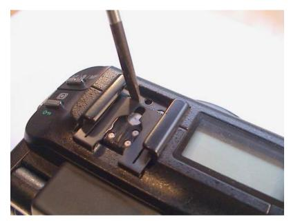
The flash cover is a little bit tricky. You have to lift up the front and then slide it out backwards. Don't use brute force!
